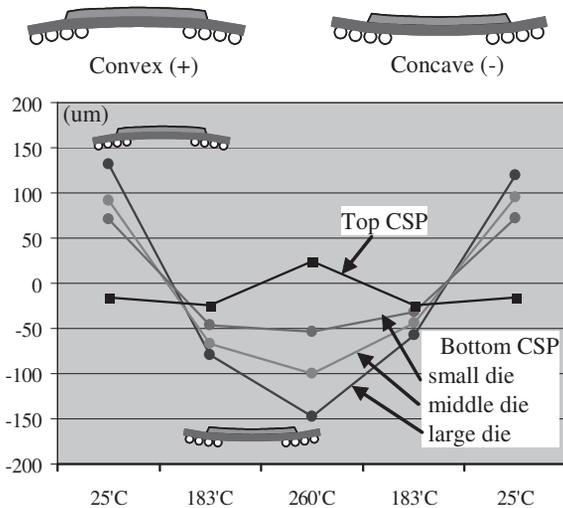
Figure 3: Warpage for the test vehicles
