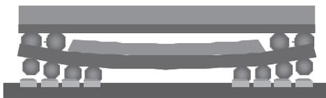
Figure 7: Mechanism of open joints
