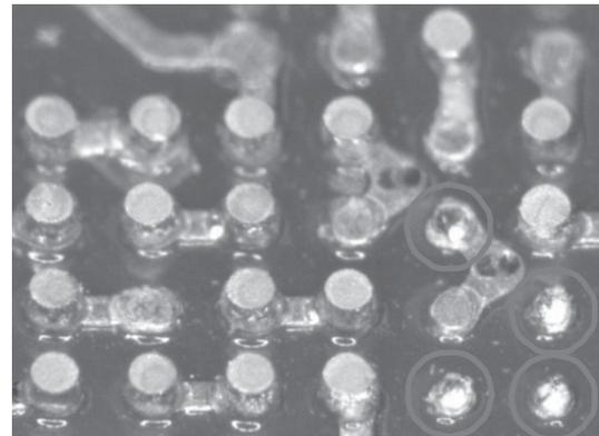
Figure 5: Open solder joints
